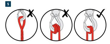
Do not twist the sling to shorten - loop the sling once instead and not multiple times
