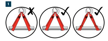
Use object extrusions or choke hitch to stop the sling slipping
